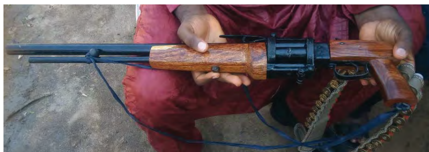
Image 6 Artisanal shotgun capable of discharging several shots successively, Nigeria, 2017
