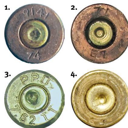
Photos 1 and 2: 7.62 × 39 mm cartridge cases produced in China Photo 3: 7.62 × 25 mm Tokarev cartridge case produced by Prvi Partizan in Serbia Photo 4: 7.62 × 25 mm Tokarev cartridge case produced in China
