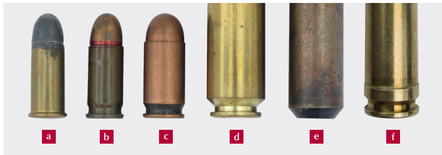
Image 4.6 Typical cartridge case rim configurations
