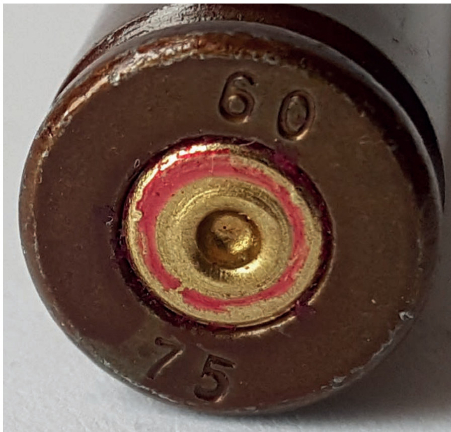
Image 4.4 Headstamp markings on a 7.62 × 39 mm cartridge case
