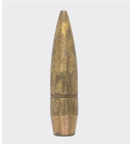
Image 4.3 A fired projectile, showing characteristic impressions left by a weapon's rifling (lands)
