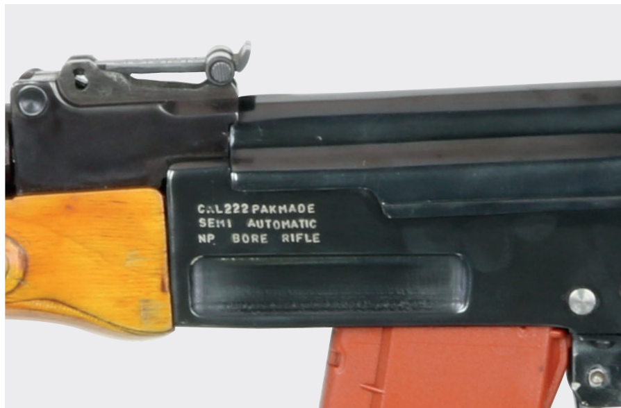
Image 6.10 Markings on an AK-type self-loading rifle craft produced in Pakistan
