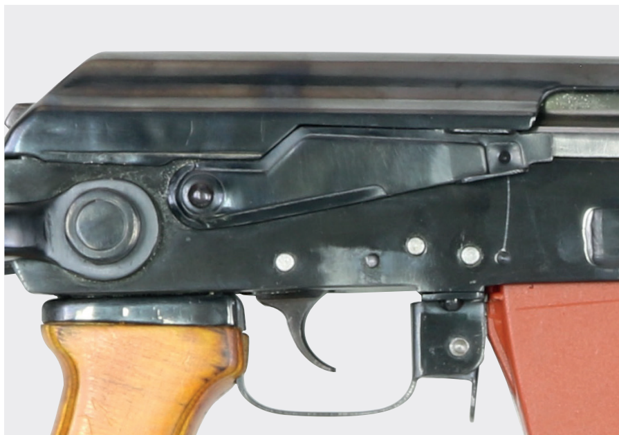
Image 6.11 An AK-type self-loading rifle craft produced in Pakistan, without the typical fire selector markings
