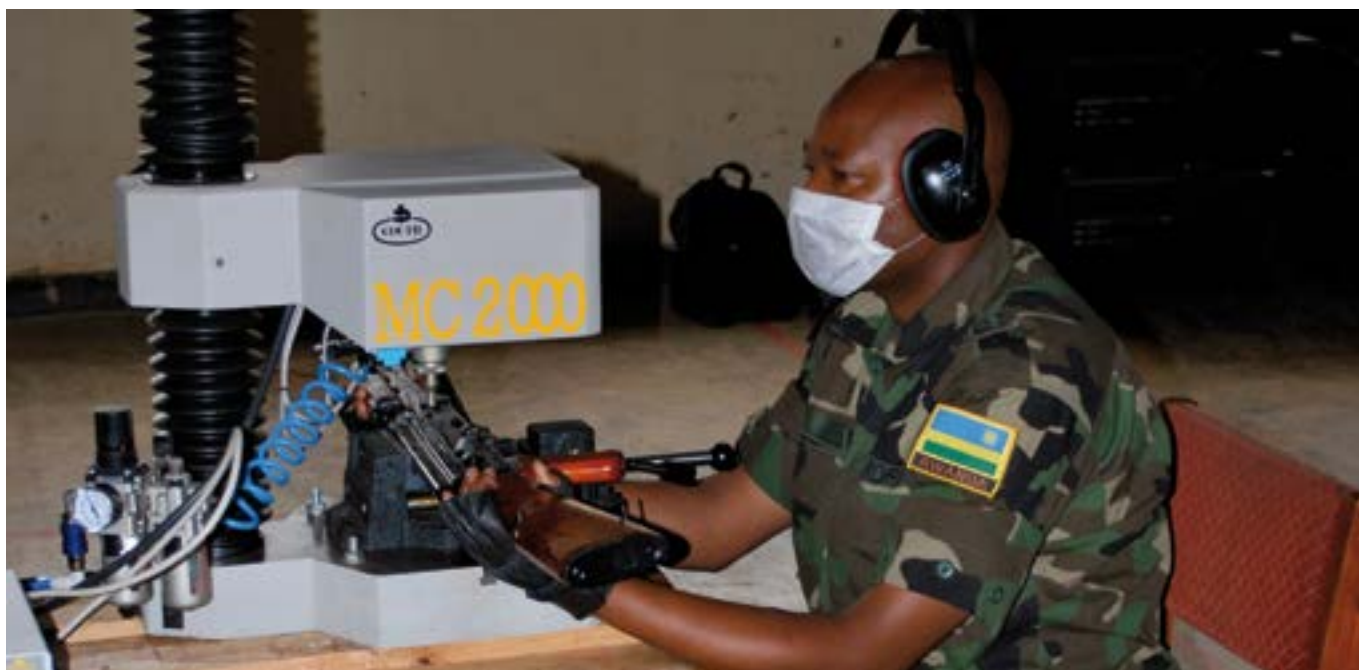
During one of many marking capacity-building projects carried out, a Rwandan Defence Force member stamps post-manufacture marks on army rifles, in Kigali, Rwanda, November 2011. © Benjamin King
