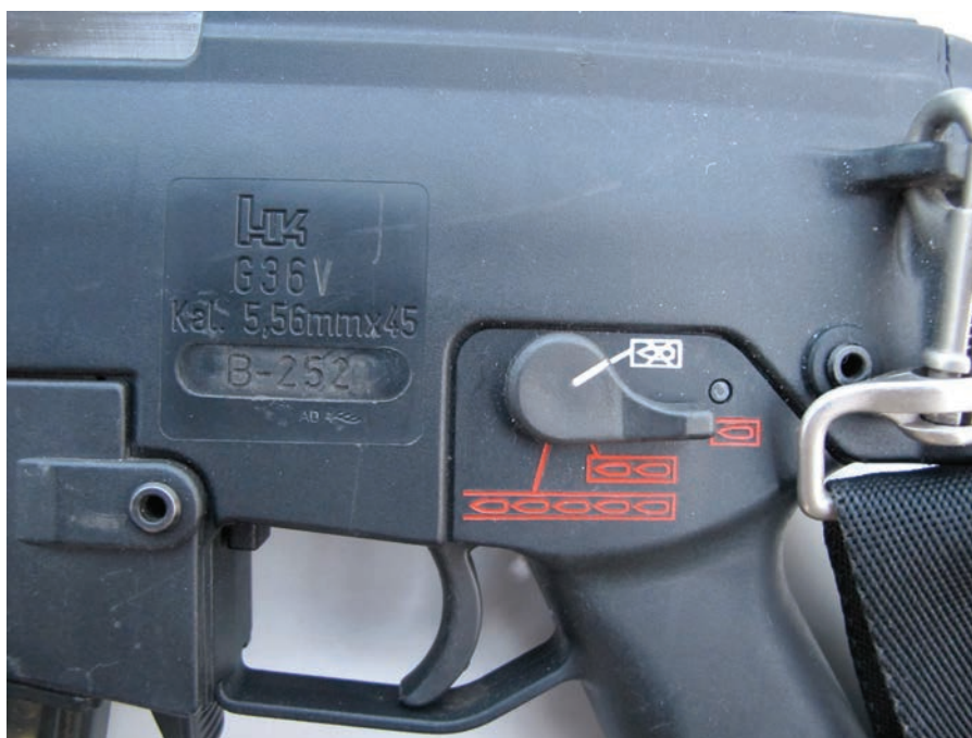
Figure 3c Weapon markings on a German Heckler & Koch G36 type self-loading rifle. Visible markings include the manufacturer marking, model designation, calibre, and fire selector marks (pictogram type). Marking that appears to be a serial number ('B-252') has been engraved over an abraded factory-marked serial number. Source: Damien Spleeters
