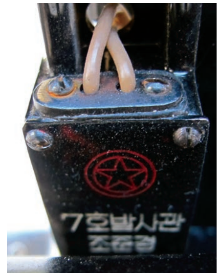
Figure 8a Markings on a North Korean copy of a PG0-7B optical sight. Source: Damien Spleeters
