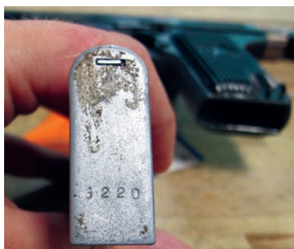
Figure 5b A partial serial number stamped on the floor-plate of a Romanian TTC 7.62 x 25 mm magazine. Source: N.R. Jenzen-Jones/ARES
