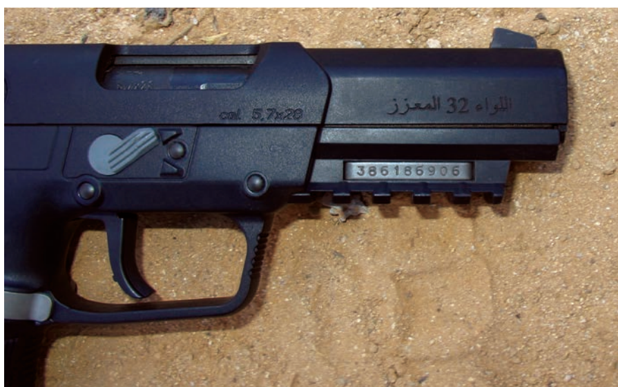
Figure 3e Weapon markings on a Belgian FN Herstal Five-sevenN self-loading pistol. Visible markings include calibre markings (duplicated in two locations), serial number, and customer-specific markings presumably applied at the time of manufacture. In this case, the Arabic text reads ‘32nd Reinforced Brigade’, referring to the Libyan Army formation to which the handguns were issued. Source: Damien Spleeters
