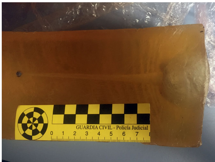
Image 4 Test firing of the impact of a ball bearing fitted into 8 mm PAK ammunition. The penetration of the projectile is considered potentially lethal. Test conducted by the Ballistics Department of the Guardia Civil. Photo taken on 19 April 2017. Source: Benjamin King/Small Arms Survey
