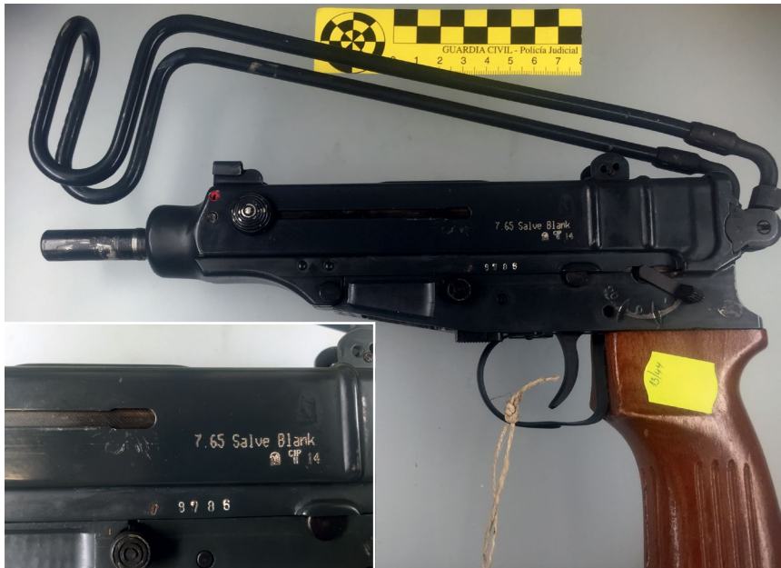
Image 3 Converted AEW seized by the Spanish Guardia Civil. Markings indicate the new ammunition requirements and proof of transformation of the vz.61 to a blank-firing AEW. Photographed on 18 April 2017. Source: Benjamin King/Small Arms Survey
