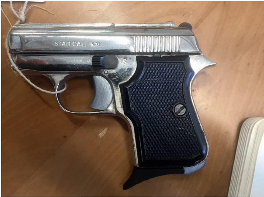
Image 1 Converted imitation Tanfoglio GT 28 alarm pistol with fake manufacturer markings and indications of new, post-conversion calibre. Photo taken at the Spanish Policia Nacional offices in Madrid, 18 April 2017. Source: Benjamin King/Small Arms Survey
