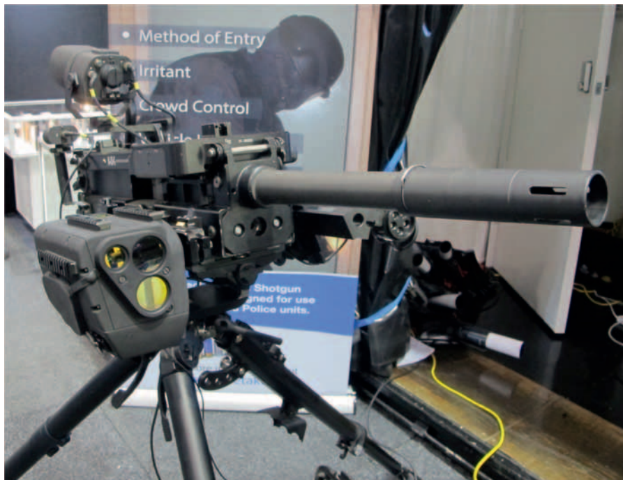
A Heckler & Koch GMG E automatic grenade launcher with Vinghøg Vingmate FCS mounted on a Softmount Combi mount. © N.R. Jenzen-Jones
