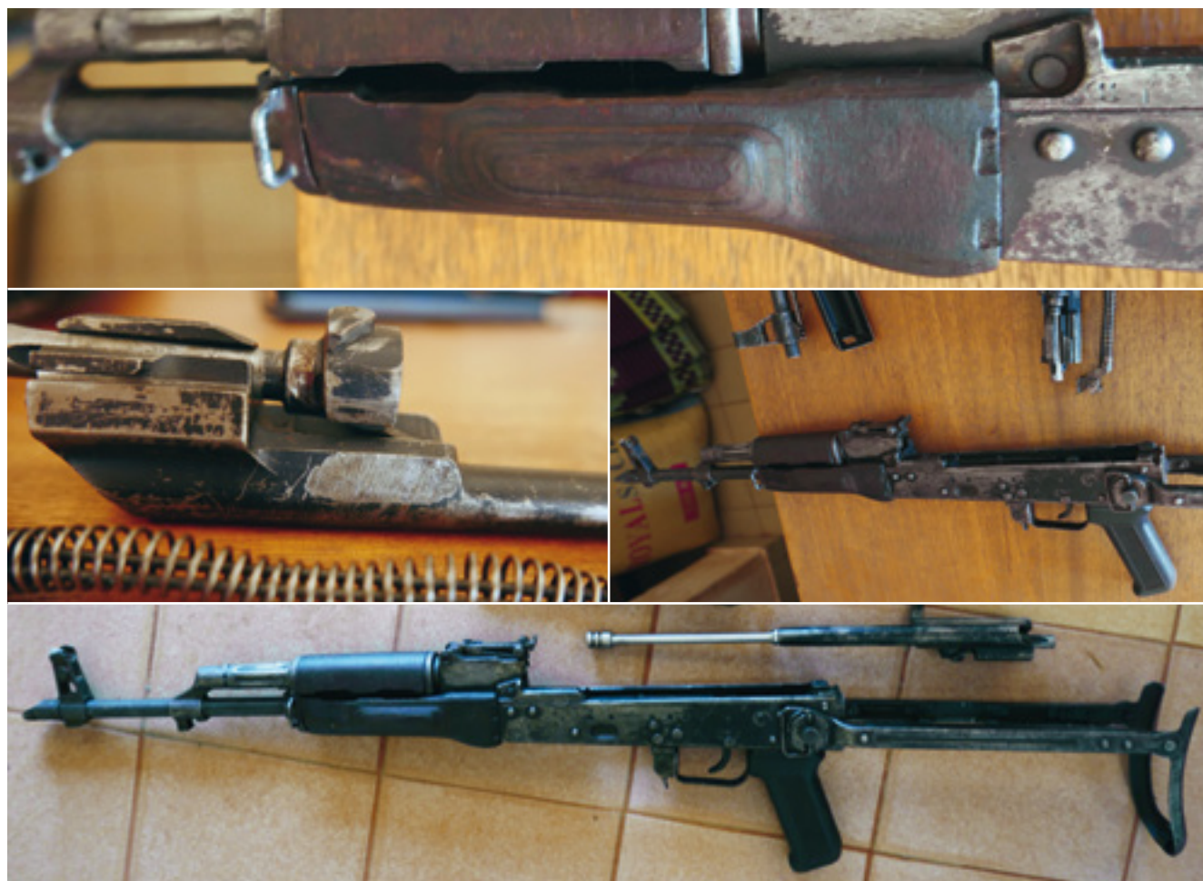
Photos 1–4 A disassembled AKMS rifle with a folding stock*
