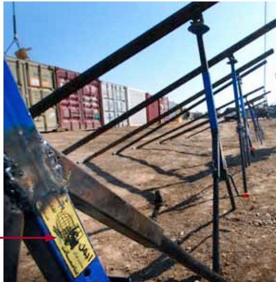
Images 8a, 8b, and 8c: Car jacks used in the construction of improvised rocket launchers, Iraq, 2008–09
