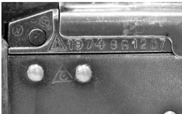
Figure 3.8 Iraqi import mark on a Russian-manufactured AKM
