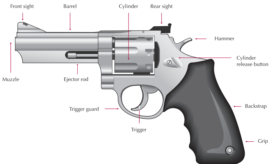
Figure 1 Parts of a handgun: revolver
