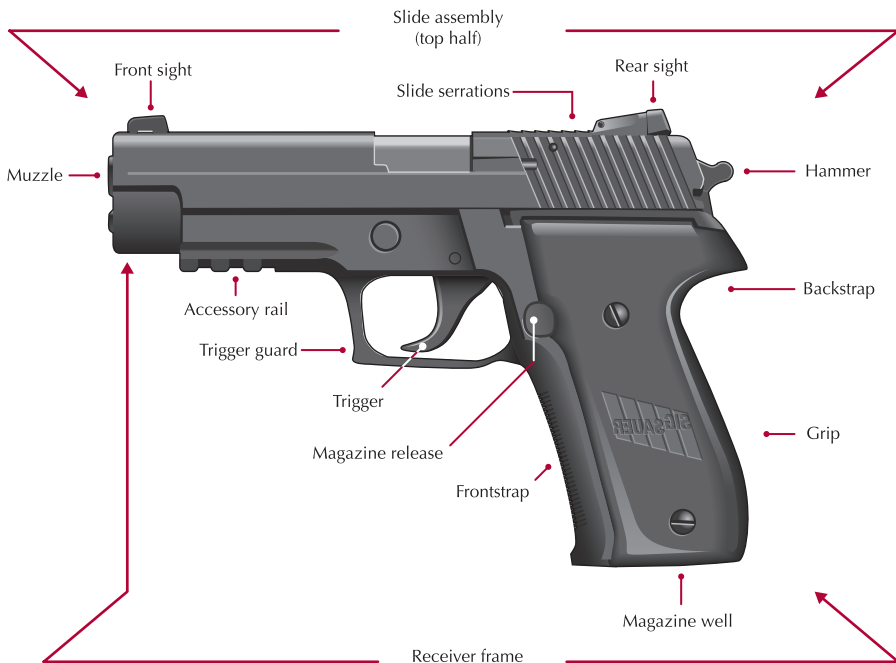
Figure 2 Parts of a handgun: semi-automatic pistol (Sig Sauer)
